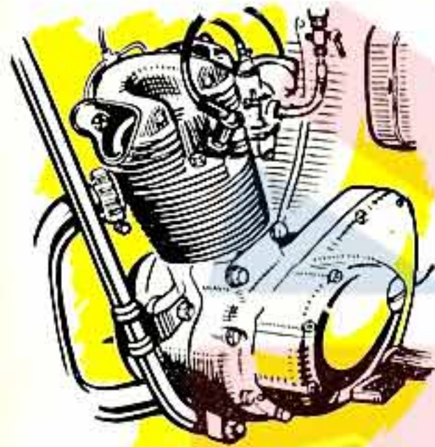
O.H.V. "Tiger Cub" engine with alloy head and unit four speed gearbox.
