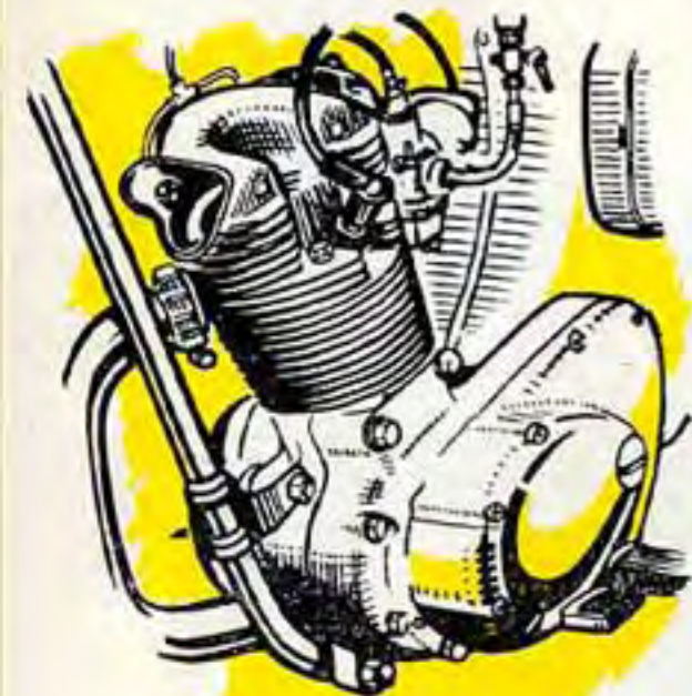
O.H.V. "Tiger Cub" engine with alloy head and unit four speed gearbox.
