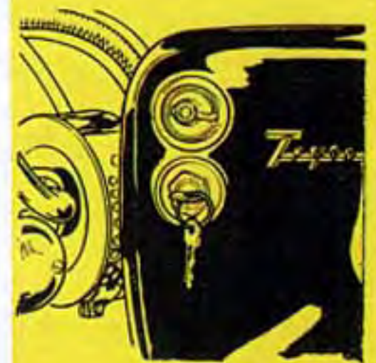
The new cylinder type Ignition Switch. Warning light fitted in headlamp.
