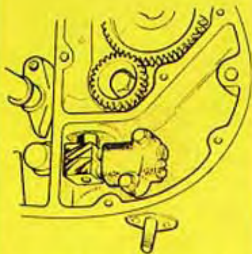
New Oil Pump of increased capacity on both feed and scavenge, with improved drive to plungers.
