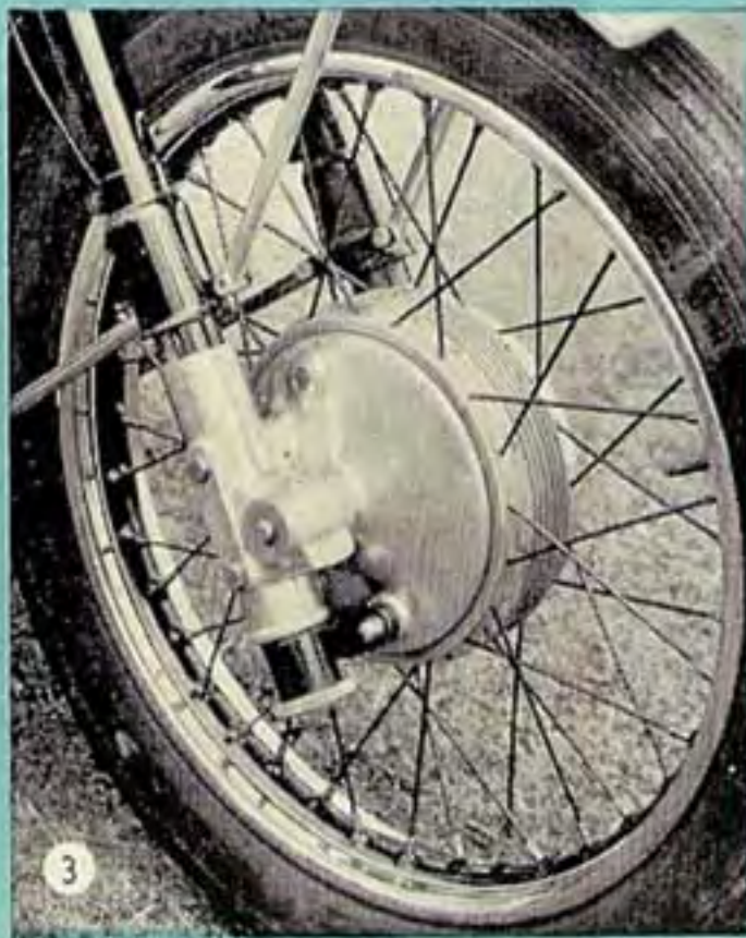
3. Front Wheel, showing Suspension System and Massive Brake Drum.
