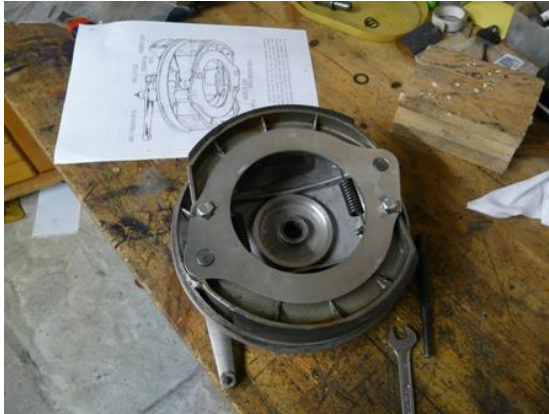
Fig.H14 Twin leading shoe brake with high performance modification
