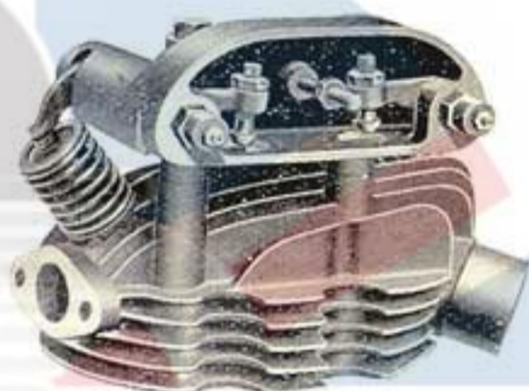
Showing cover of O.H.V. Rocker gear with inspection plate detached.
