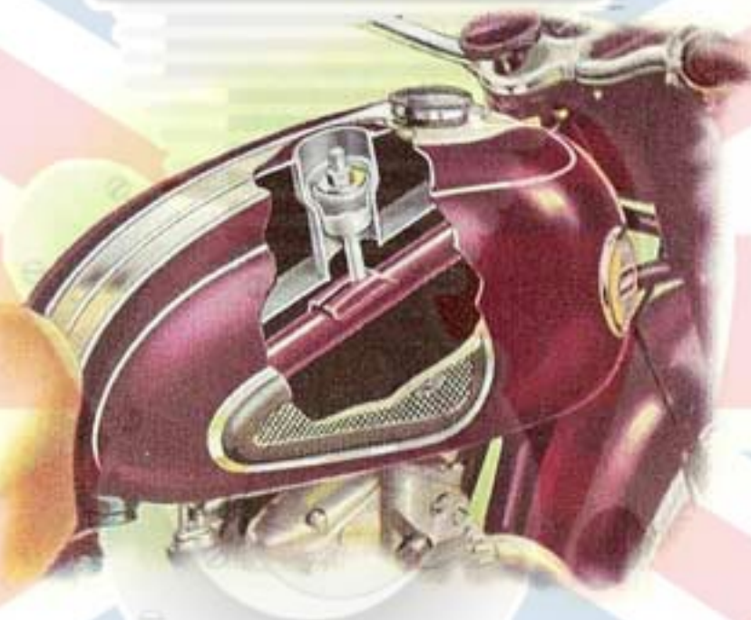
New single bolt fixing petrol tank for all swinging arm models.
