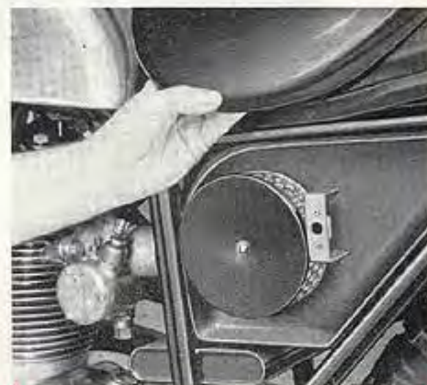
The double-paper element air cleaner in fibreglass case with the quickly-detachable cover removed. Note oil header tank immediately below air cleaner casing.
