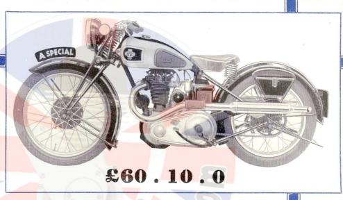
BORE & STROKE-70 m.m. 90 m.m. 346 c.c. Two-port compressed head. High lift cams.
