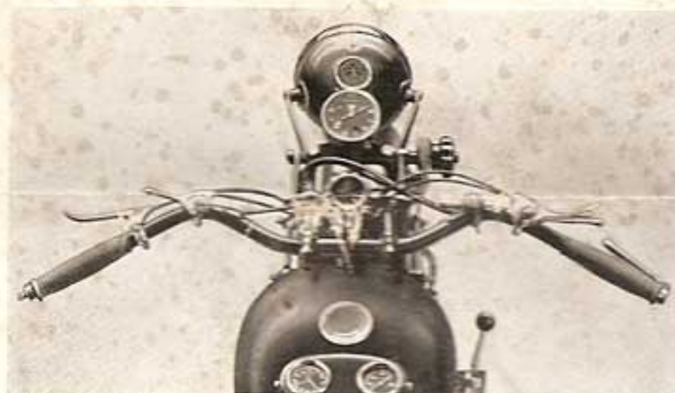
INSTRUMENTS and CONTROLS. Instruments arranged so that they can be seen by rider, without taking his attention from the road. Controls adjustable to suit rider's requirements.
