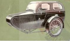
FAMILY SIDECAR Model S23-52. Finished in black. This is the sidecar for the family man. It provides saloon-car comfort for an adult and child. It is completely weatherproof. The top of the body hinges towards the machine for easy access. Leg room 51°, seat width at elbows 21°. Height inside 32°. £70 10s. plus £16 7 10 tax
