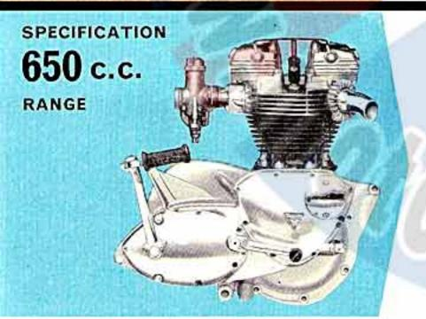
ENGINE. 650 c.c. o.h.v. vertical twin with two gear driven camshalts. Light alloy cylinder head, cast-iron barrel, high compression pistons large bore carburetter. Splayed port head with two carburetters on T120. Finned rocker boxes. One-piece forged crankshaft with bolt-on central flywheel. "H" section RR56 alloy connecting rods with plain bearing big-ends. Dry sump lubrication with plunger type pump and pressure indicator. Twin coil ignition. Oil bath primary chaincase. Air cleaner (not T120).
