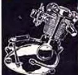
THE TIGER CUB UNIT CONSTRUCTION ENGINE AND GEARBOX.
