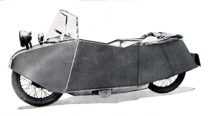
The beautiful clean streamline shape of the Whitwood accounts for the high performance and economical running. The very full surrounding protection to all vital parts and also to the human load is obvious. The side doors are fitted with quick detachable screens which open with the doors, and are neatly lowered in a special pocket when not in use.
