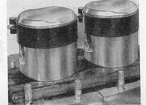
Apply a coating of clean engine oil to the pistons and position the ring gaps equally round the pistons.
