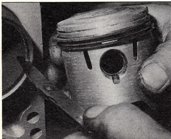
MkII pistons had the "Top Hat" shaped crown, peculiar to this model.
